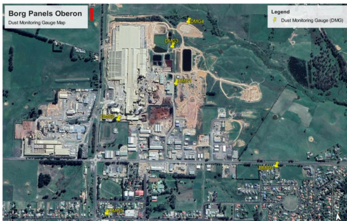
DMGs 1 to 4 are located on the periphery of the site. DMG 1 is located within the operational boundary of the site immediately adjacent to an unsealed laydown area and in general proximity of an unsealed road. DMG 2 is located adjacent to the materials handling building. DMG 4 is located towards the northern boundary in an area of unsealed compacted surfaces used for storage of large pieces of machinery and reusable material such as steel.
