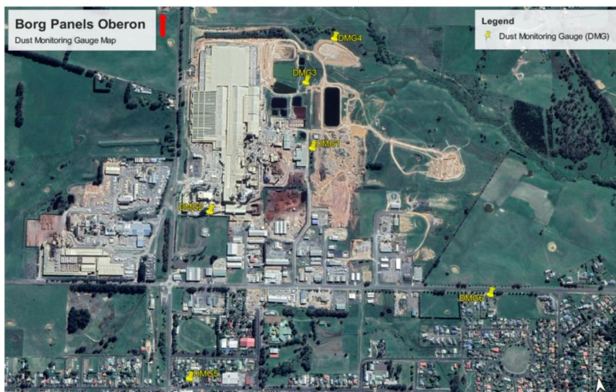
DMGs 1 to 4 are located on the periphery of the site. DMG 1 is located within the operational boundary of the site immediately adjacent to an unsealed laydown area and in general proximity of an unsealed road. DMG 2 is located adjacent to the materials handling building. DMG 4 is located towards the northern boundary in an area of unsealed compacted surfaces
