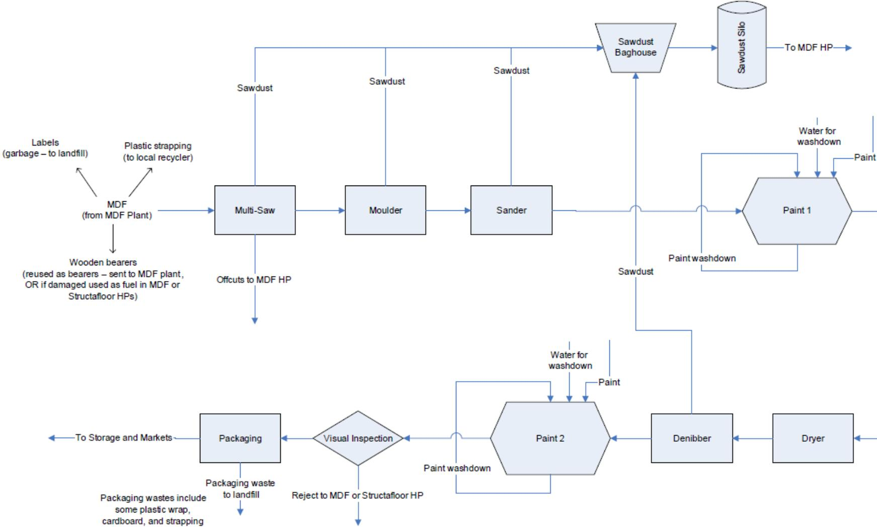
Figure 2 – Schematic Overview of the Mouldings Production Process
