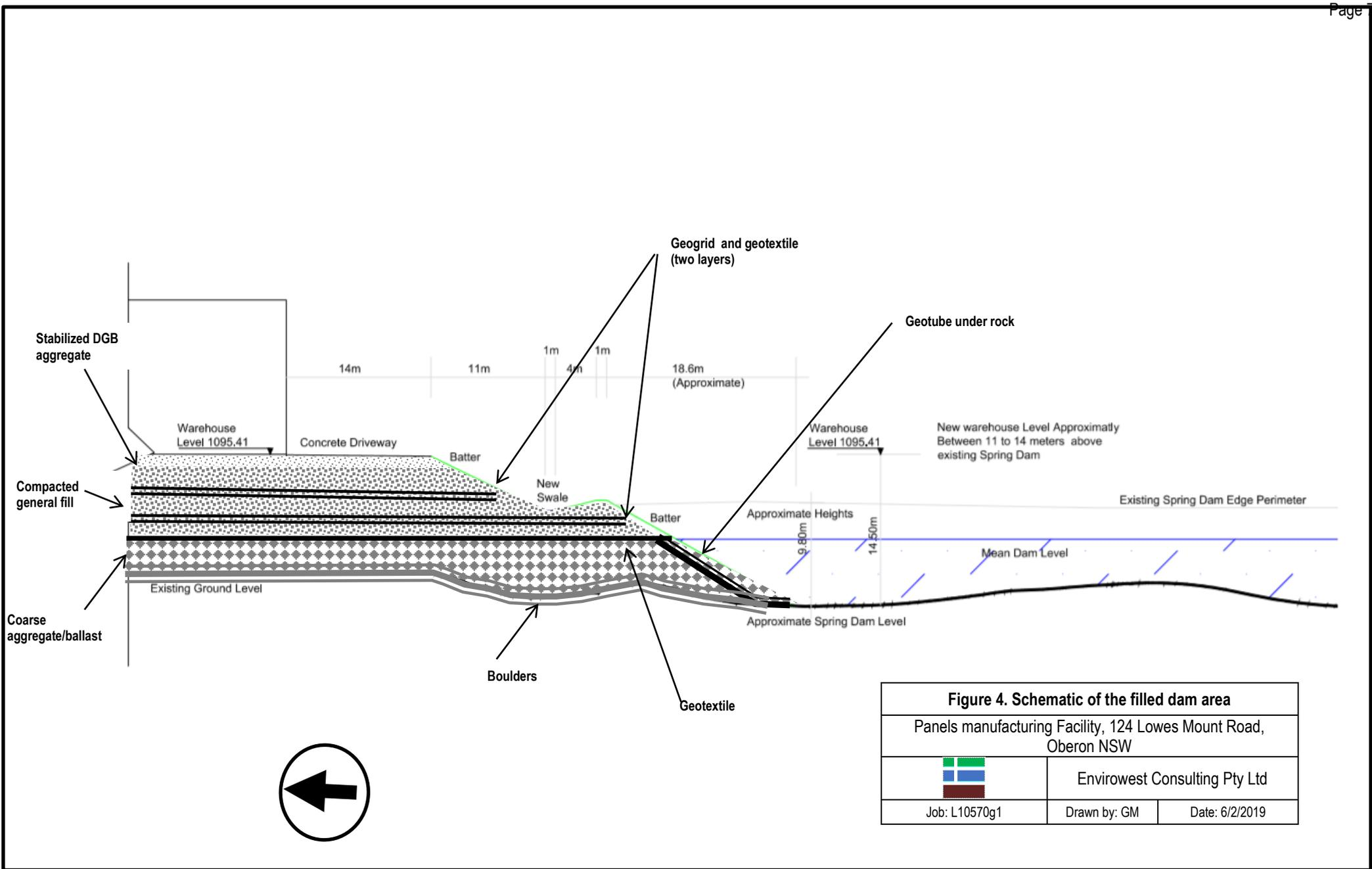
**Figure 4. Schematic of the filled dam area**
